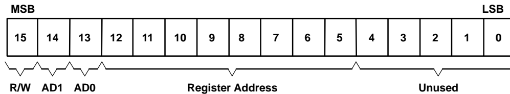
Figure 5. Bit Assignment and Definition for Slot 0 Word
